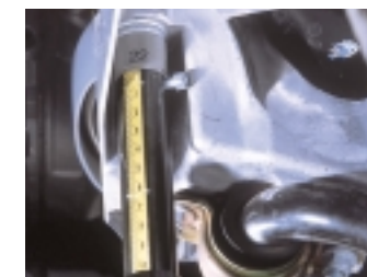
Measuring tube and adapter fits over bolt head in tight places.
