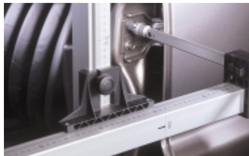
Upper body measuring points are easy to reach with the M900 upper body measuring system.
